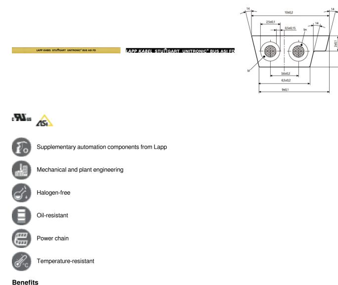
The new BUS ASI LD 2 x 2.5 (Long Distance) allows even modules located further away to be connected. AS-I power supplies can be reduced. The BUS ASI LD is downwards-compatible with version 1.5. For highly flexible applications (power chains, moving machine parts) High oil-resistance
