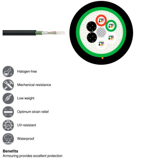
Armouring provides excellent protection against high mechanical stress and rodents Suitable for direct burial Easy to install due to the compact design, high flexibility, robust sheath and small bending radii UV-resistant longitudinally and laterally watertight
